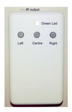
The TL-Lite is a Intervalometer or time lapse timer for Sony's range of IR enabled cameras. The TL-Lite measures (65x35x24mm) weighs 30 grams and is powered by one 3 volt CR2032 battery. Battery life over 300 hour's continuous use with the unit set at one shutter trigger every 4 seconds.
